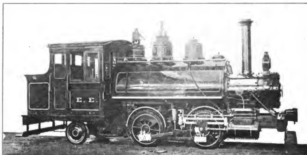
Fig. 9. Four-Coupled (0-4-2) Tank Locomotive with Trailing Truck. Built by the Baldwin Locomotive Works for the Embreeville Estate. Cylinders 10 in. x 16 in., Working Steam Pressure 100 lbs. per sq. in., Heating Surface 340 sq. ft., Diameter of Drivers 36 in., Weight on Drivers 32,440 lbs., Total Weight 37,140 lbs.
